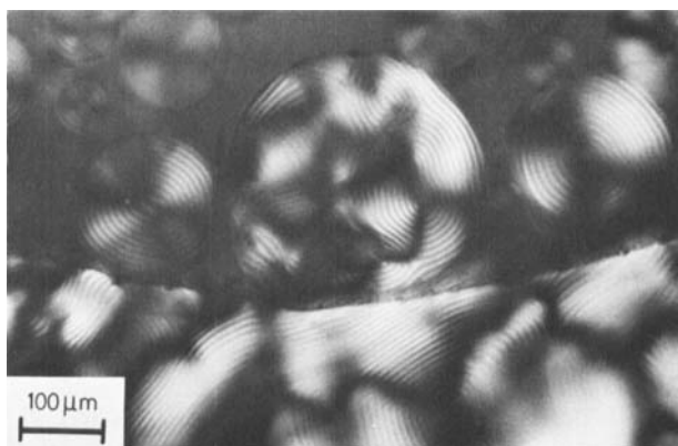
FIGURE 6 Two-phase solution of D-40 with w = 0.101 at 30^{\circ}\text{C} .
